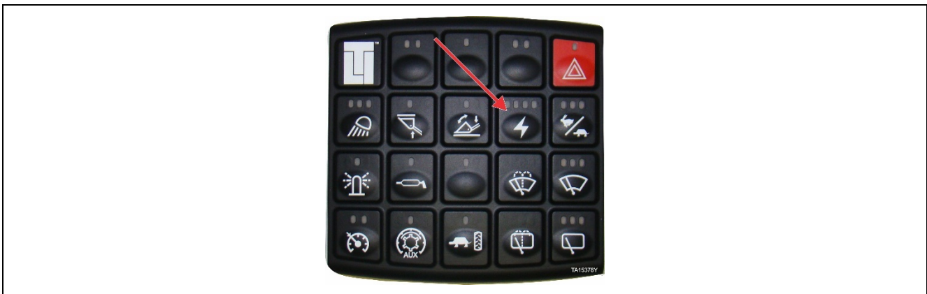
Figure 32. Drive Enable Switch
