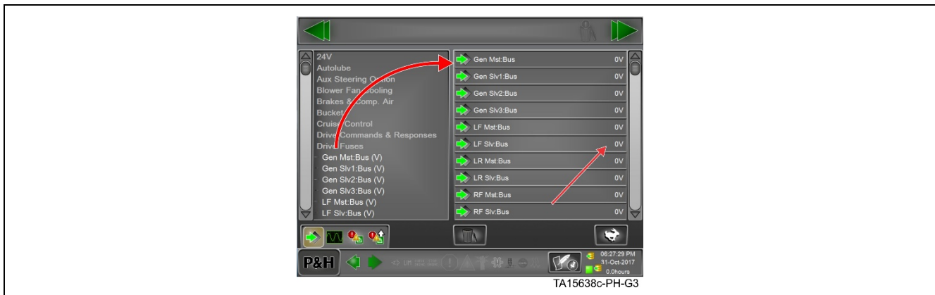
Figure 22. Bus voltage indication
